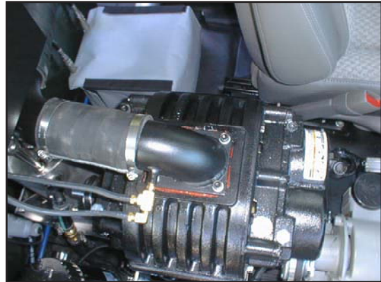
Figure 7. Install Blower Power Pack, Clutch Mounting Bracket, Clutch and Position Salsa Heat Exchanger
