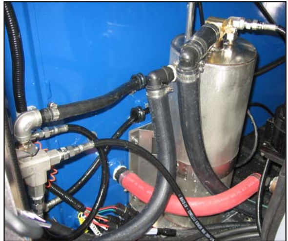
Figure 8. Connect Hoses to/from Coolant Heat Exchanger
